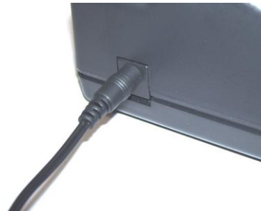
12V Power Supply Connected to Power Jack
