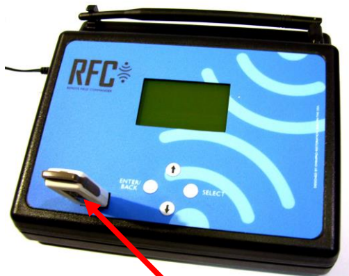
Flash Drive inserted into USB port to download job data.
